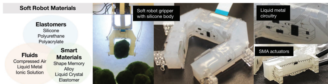
Figure 3. Soft robots are typically composed of elastomers, fluids, and smart materials that respond to electrical or thermal stimulation. An example of this is a soft robot gripper that has a silicone elastomer body, liquid metal circuitry to support embedded microelectronic components, and shape memory alloy for electrical actuation. Reproduced with permission. [15] Copyright 2018, Institute of Electrical and Electronics Engineers.
