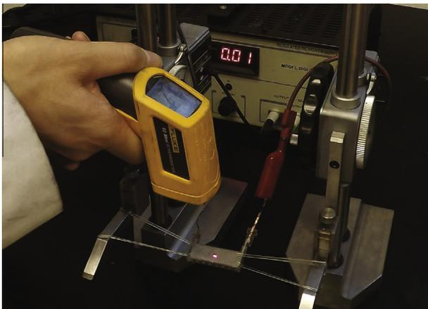
Fig. 4. Experimental setup for the surface temperature history measurement.
