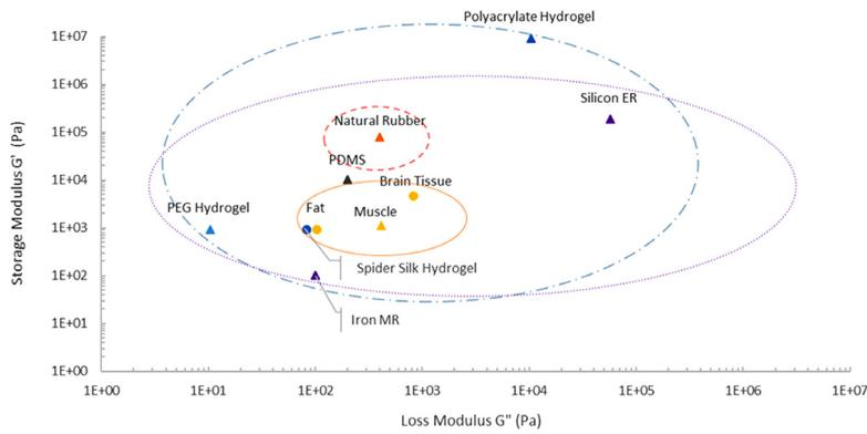
**Fig. 1.** Approximation of Storage Modulus vs Loss Modulus of various organic and inorganic materials. Hydrogels: - - -; Biological Tissue: ——; Natural Rubber: - - -; Electrorheological (ER) And Magnetorheological (MR) Fluid Based Polymers: .....; Materials that have been used in soft robots: Triangle; Hard Materials: Diamond.
