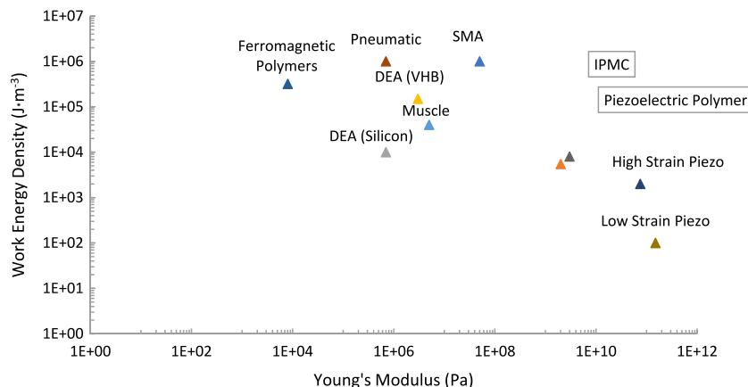
**Fig. 2.** Work Energy Density vs Young's Modulus of established soft robotic actuator technologies [10,18,19]. Abbreviations: SMA – shape memory alloy, IPMC – ionic polymer-metal composite, DEA – dielectric elastomer.
