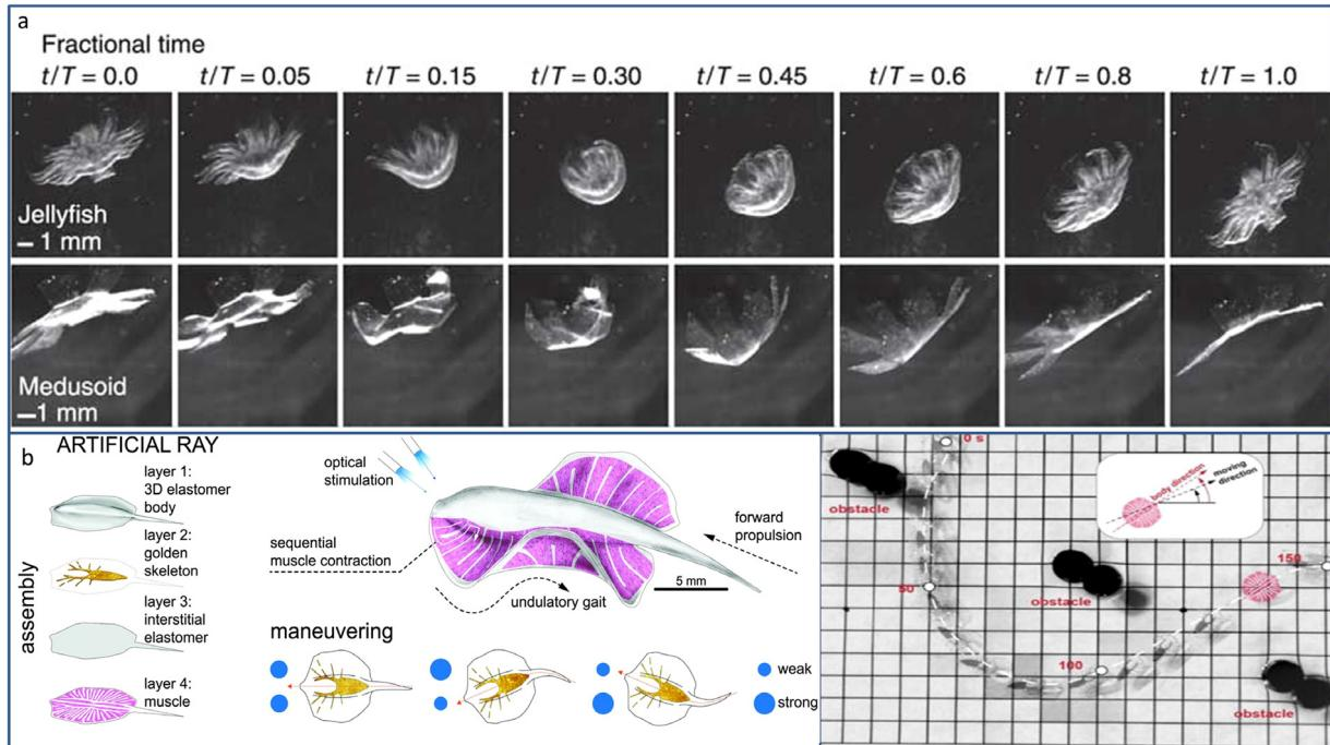
**Fig. 5.** Biohybrid muscle cell based actuators (a) Time lapse of stroke cycle in jellyfish (top) and an artificial jellyfish (bottom) [90], (b) (left) A biohybrid assembly components that mimics the actuation behavior of a sting ray, (b) (right) Soft artificial ray navigates through an obstacle course [93].
